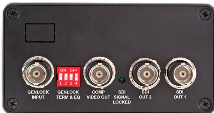
The two right hand BNC’s both provide a digital HD output. The LED shows a solid green colour for a valid HD-SDI signal being present.
