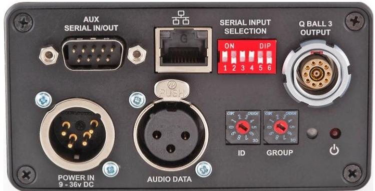
The left hand rotary switch should be set to the required ID number being used by this camera. Normally this will be in range 1-8 to agree with the channel selected on the RCP and PTZF controller. The right hand rotary switch sets the ID Group No. This allows extending the number of possible units being controlled using the Camera Corps Multi Camera control system to a maximum of 96.
