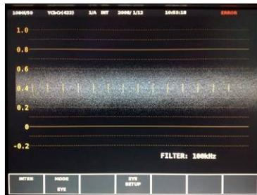
1.485Gb/s serial digital signal after re-clocking with Camera Corps multi-rate re-clocker
